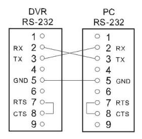
The transmission protocol is 8 data bit: 1 start bit, 1 stop bit and no parity. Five different speeds can be used: 1200 baud per second, 2400 baud, 4800 baud, 9600 baud and 19200 baud. The default setting is 2400 baud per second.
